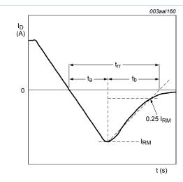
Fig. 16. Reverse recovery timing definition
