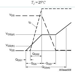
Fig. 12. Gate charge waveform definitions
